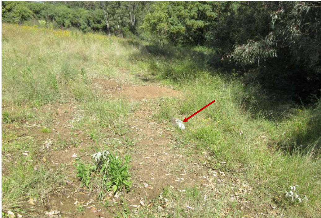
Photo 6 - Sandstone boulders partially buried within the slope (inferred colluvial soil).
